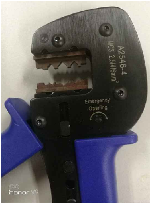
CRIMPING TOOL(CA-AES-CT-18) DIE INSERT AND CRIMPING LOCATOR INCLUDED FOR 10, 12, 14 AWG
